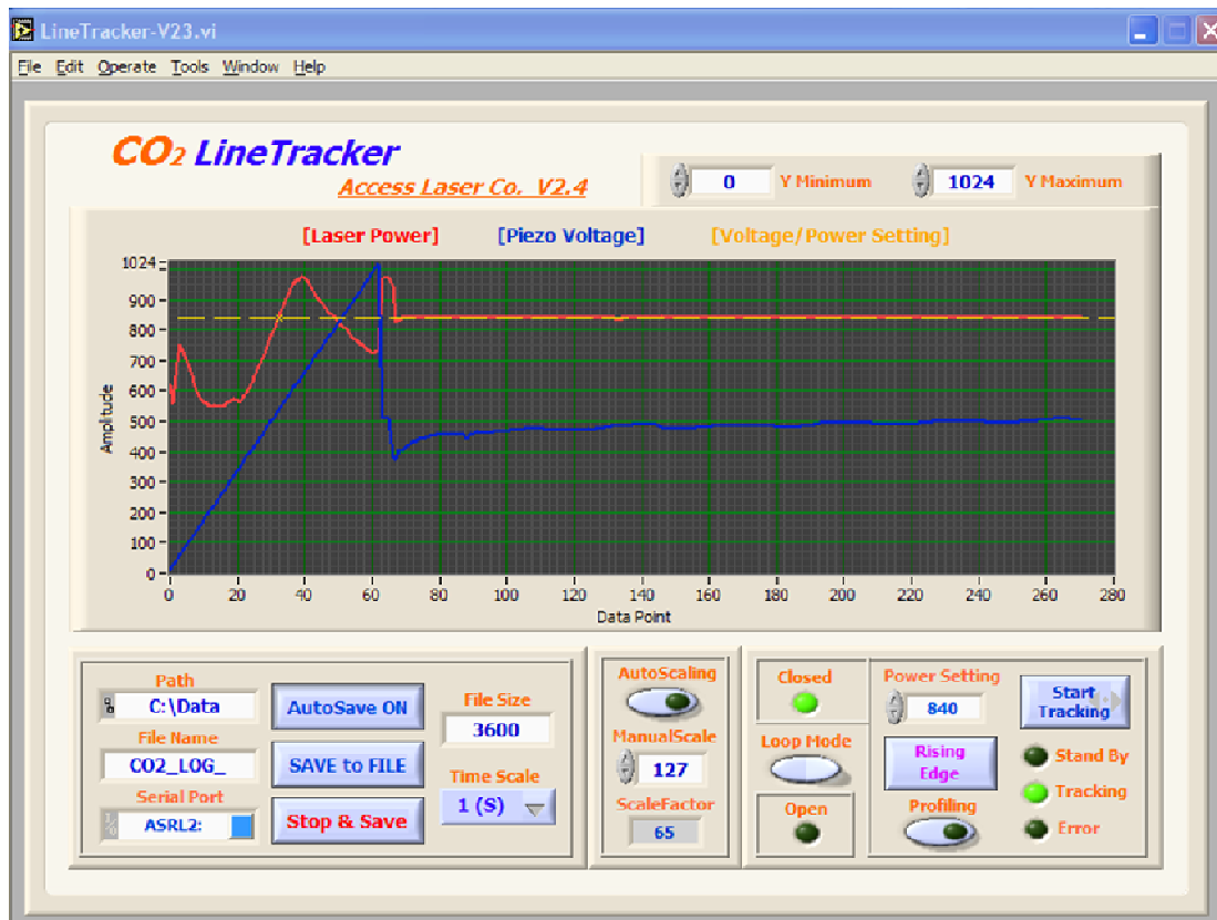
Screen shot of the Line Tracker computer interface. This plot was obtained with a Merit laser.
